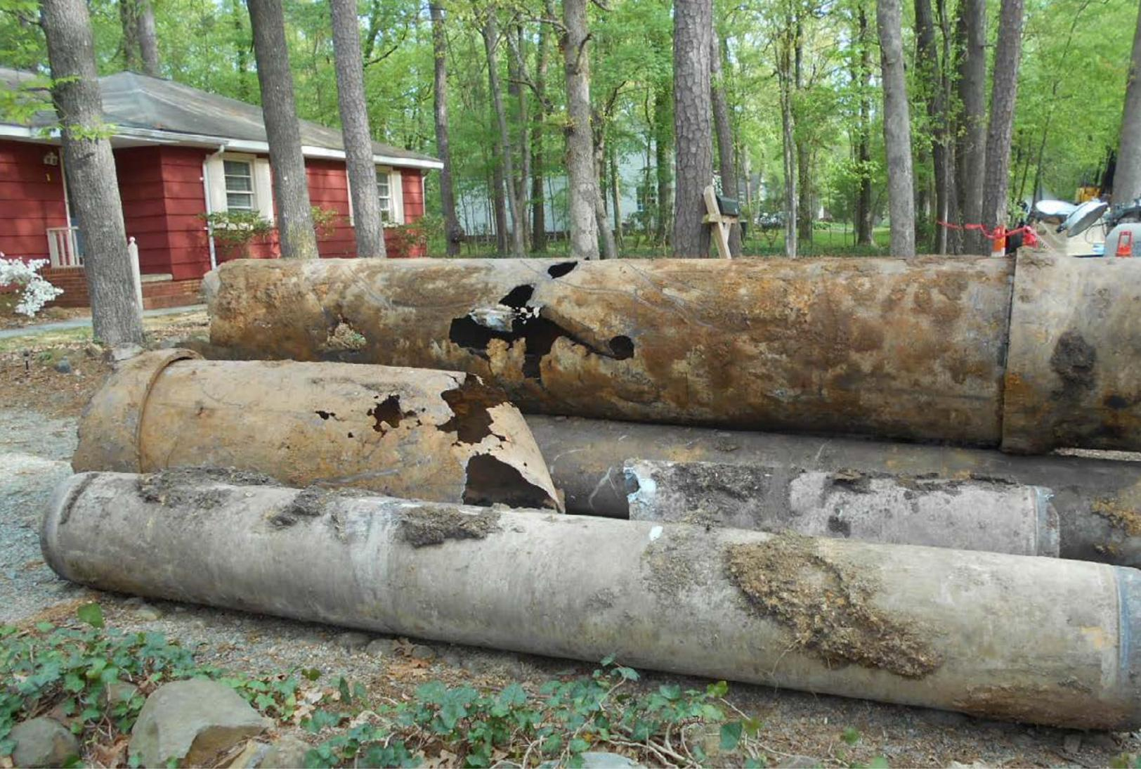
**McKim & Creed helped the Orange Water and Sewer Authority in North Carolina repair a 30-inch force main that failed due to corrosion.**
