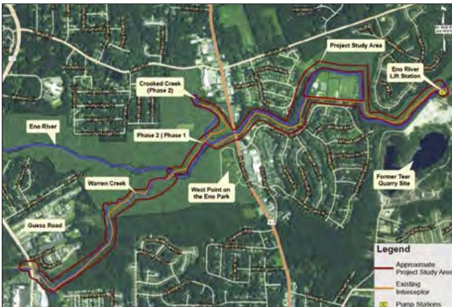
This shows the 3-mile-long project area. On the east end is the Eno River Lift Station, the City's largest. This station collects sewer generated by about 35 square miles of land, and ultimately pumps to the North Durham Water Reclamation Facility. Going west, upriver, the corridor goes through three different neighborhoods, crosses US Highway 501, then traverses mostly through parkland before crossing NC Highway 157 at the westernmost end.
